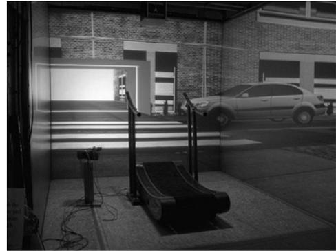
Figure 1. The street crossing simulator in the CAVE at the Beckman Institute Illinois Simulator Lab.
